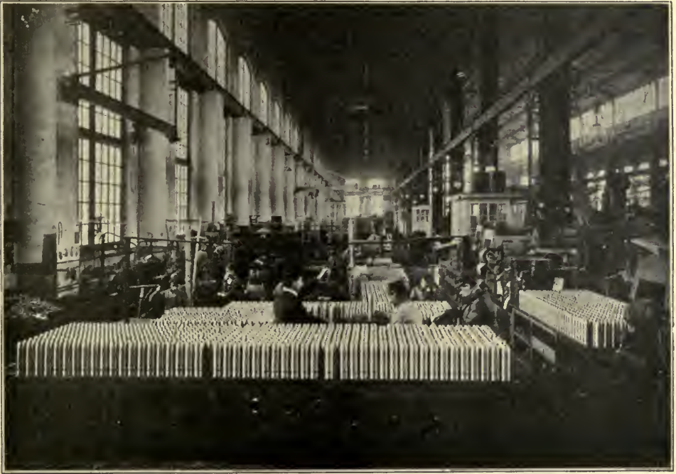
INSPECTING SHELLS FOR "SEVENTY-FIVES" AT LE CREUSOT
